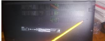
Simply unfold the paper clip, insert the straight edge to press the button inside until the laptop powers off:
